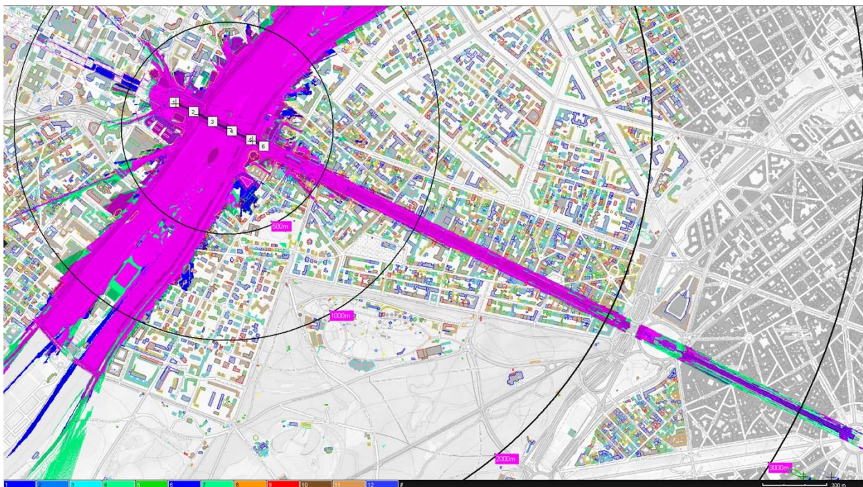
Figure A.14: Paris L1 - Common and additional Protected Zone between car (antenna height = 1,7 m) and truck (antenna height = 4 m) for Road-ITS 33 dBm EIRP and CBTC DSSS with 3 dB desensitization
