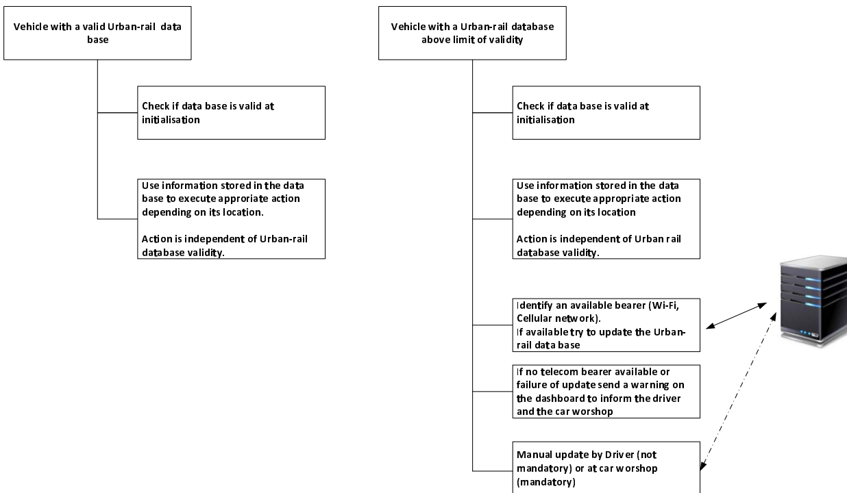
Figure E.3: Process for phase two expected behaviour of a road vehicle
