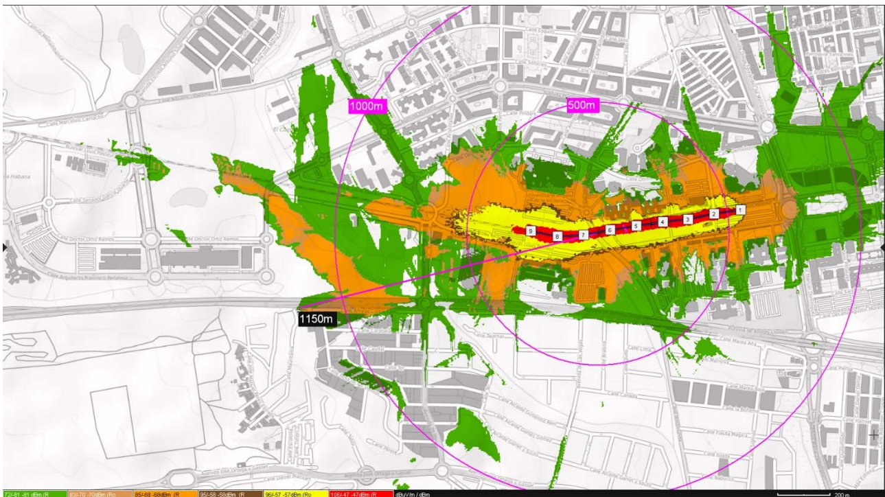
Figure 17: Adjacent channel impact - Train Protected Zones for different scenarios of Road ITS EIRP with antenna height 1,5 m and different CBTC systems and radio planning rules
